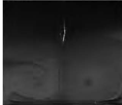
Fig. 3 Visualization of Ionic Wind Flow
